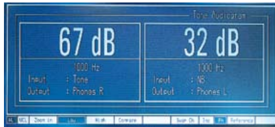
Large digits are preferred by some users and are therefore provided as an alternative to displaying audiograms.
